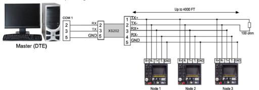
Notice: The remote RS232 end needs to be connected to a standard RS232 port. A loopback test will not work in this extension setup.
